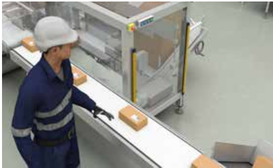
Point of operation guarding
