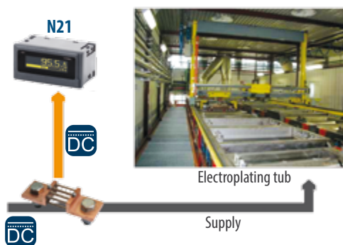
Current measurement in an electroplating plant
