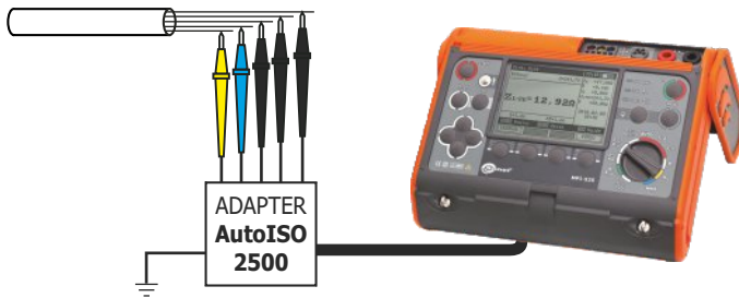
Fig. 9. Measurement of insulation resistance in multi-core cables using the AutoISO-2500 adapter.
