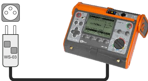
Fig. 8. Insulation resistance measured in a power supply socket with a UNI-Schuko plug (MPI-520).
